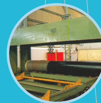
BITUMINOUS COATING SECTION
